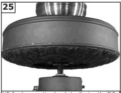
Lift fan to mounting bracket, aligning the "L" shape holes on the canopy with the screws on the mounting bracket. Turn the fan clockwise to lock in position. Re-install the screws removed in the previous step and tighten securely.
